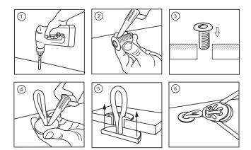
Drill a hole for the TDP. Clean the installation area with acetone to remove dust and grease. Apply Sikaflex 291i or other adhesive to make the installation watertight. Apply pressure to the product to secure it to the installation area. Attach the SLR to the loop. Wait 24 hours before putting any load on the product.
