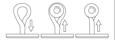
Stretch the loop open and slide in the SLR. Close the loop to lock the SLR in place.
