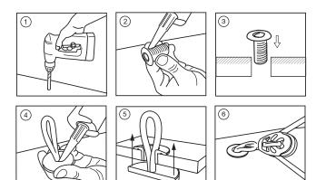
Drill a hole for the TDP. Clean the installation area with acetone to remove dust and grease. Apply Sikaflex 291i or other adhesive to make the installation watertight. Apply pressure to the product to secure it to the installation area. Attach the SLR to the loop. Wait 24 hours before putting any load on the product.
